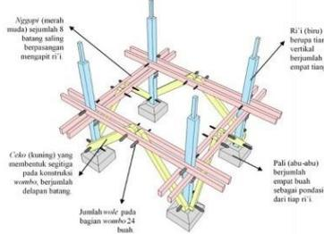
**Gambar 4.** Konstruksi Wole Uma Jompa
