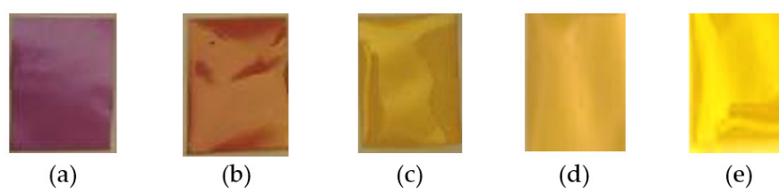
Figure 1. Appearance of the polymer film sample with 20% TCE after radiation with doses of (a) 0 kGy; (b) 2 kGy; (c) 4 kGy; (d) 6 kGy; and (e) 12 kGy.
