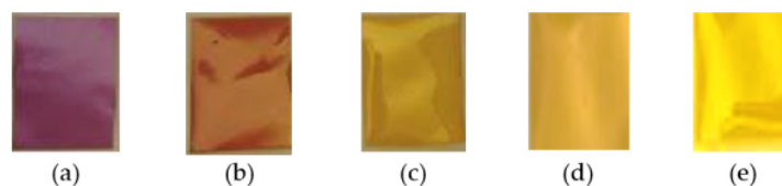
Figure 1. Appearance of the polymer film sample with 20% TCE after radiation with doses of (a) 0 kGy; (b) 2 kGy; (c) 4 kGy; (d) 6 kGy; and (e) 12 kGy.
